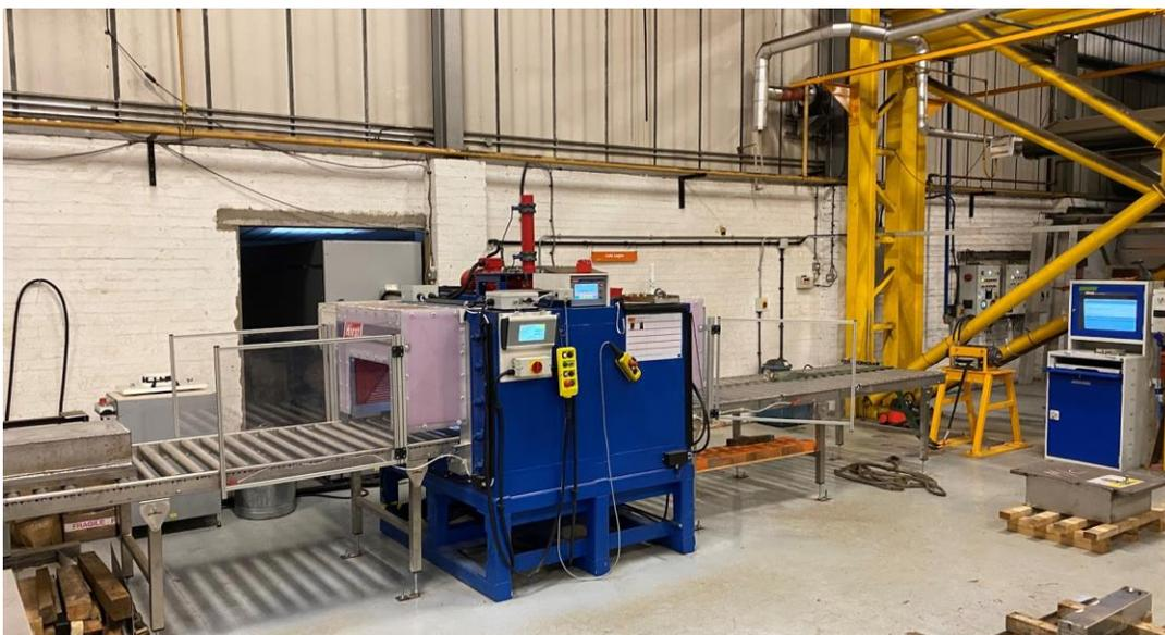
As pictured, this specialised charger works by passing a 300kj high intensity current from the capacitor bank through an unmagnetised block of Strontium ferrite or Neodymium iron boron. This ensures that all blocks are consistently
