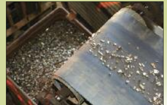
Nonferrous fines drop into collection bins.
