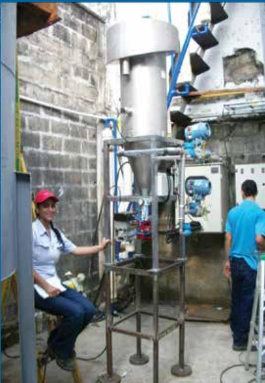
Figure 1: A 16 inch diameter small-scale production HydroFloat™ for gravity tails flotation
